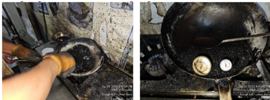
Figure 12. Wet Mixing (90-120 seconds)
