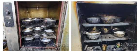
Figure 9. Kiln for heating aggregate
