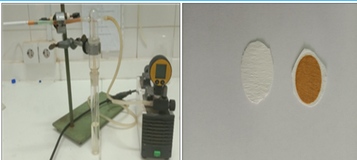
Figure 1. A- Smoking Manual Machine, B- GF Paper Used to Trap Nicotine.
