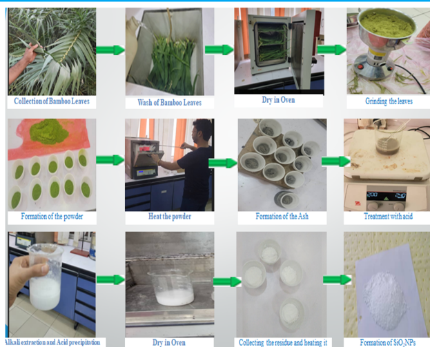
Figure 2. Green Synthesis of Silica dioxide Nanoparticles from Bamboo leaves ash.
