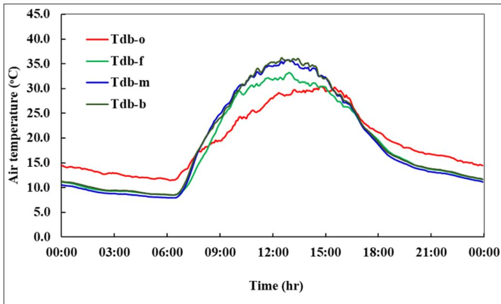
**Figure 3.** Diurnal variation in air temperature inside a plastic-covered greenhouse. Tdb-o represents the outside air temperature, while Tdb-f, Tdb-m, and Tdb-b indicate the air temperature in the entrance, middle, and end sections of the greenhouse, respectively.
