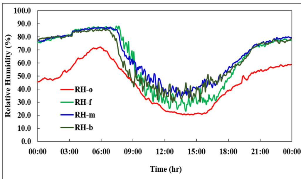
**Figure 4.** Diurnal variation in air relative humidity inside a plastic-covered greenhouse. RH-o represents the outside relative humidity, while RH-f, RH-m, and RH-b indicate the air relative humidity in the entrance, middle, and end sections of the greenhouse, respectively.
