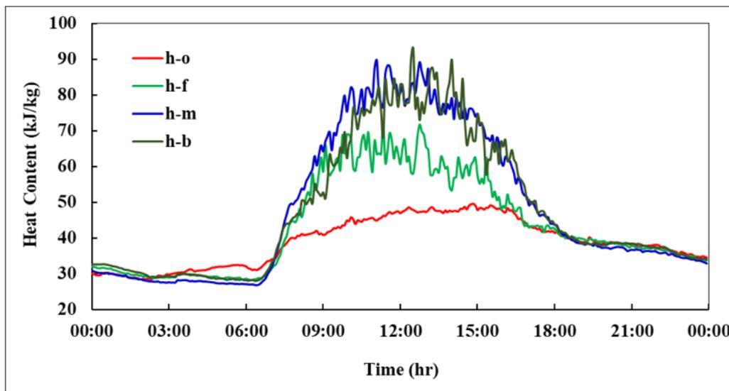
**Figure 6.** Diurnal variation in air heat content inside a plastic-covered greenhouse. h-o represents the outside heat content, while h-f, h-m, and h-b indicate the air heat content in the entrance, middle, and end sections of the greenhouse, respectively
