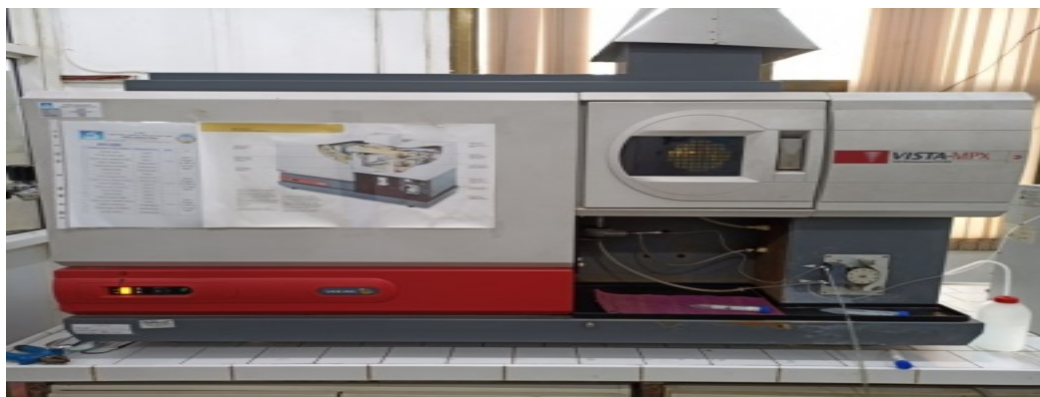
Figure 5. (ICP - OES) device for heavy metal concentration analysis.
