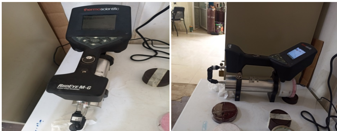
Figure 6. Gamma spectrometer Nal (TI) Thermo Scientific RIIDEYM-G
